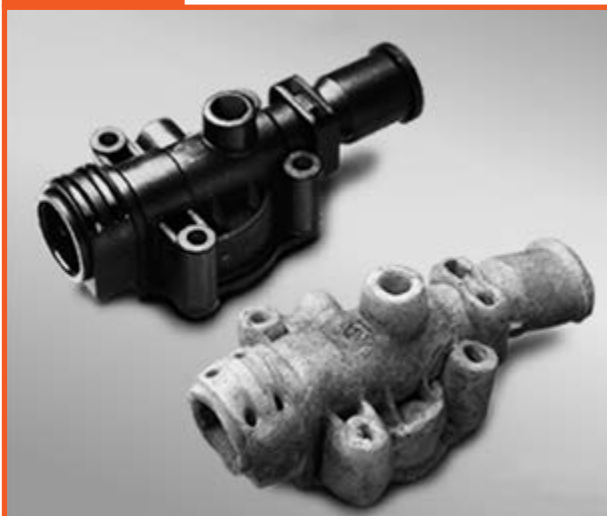
After burning off, a molding (example: pump head made from Celstran® PA66-GF50, top) retains its geometry almost intact as a fiber skeleton (bottom)
